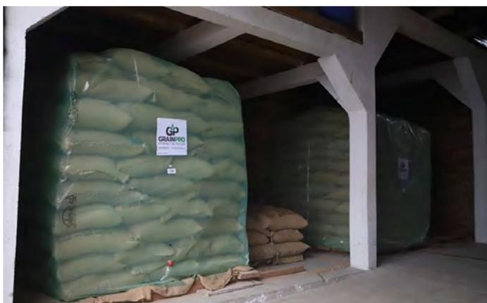
Indoor airtight grain storage cocoon manufactured by Grain Pro
