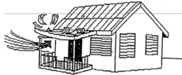
Light weight verandah roofs are more susceptible to damage by high speed winds.
