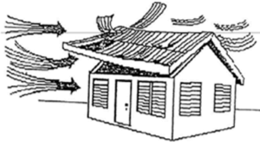
Roofing materials not anchored can be blown away.
