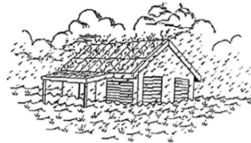
When cyclones are accompanied with heavy rain for a long duration, the building can be damaged due to flooding.
